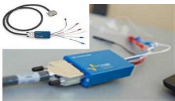
Photo 2. Ultra-Low-Current Sonde in the range 1pA - 500mA.
